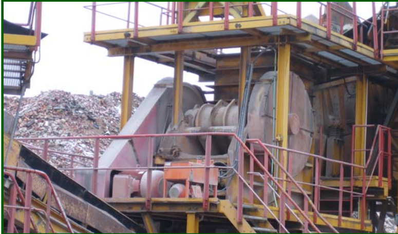
Jaw crusher 1,200 x 900 mm throughput 120 – 180 m 3 /h
