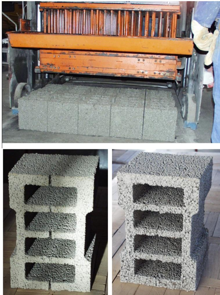
**Fig. 19.** Production of lightweight concrete blocks, left concrete block of lightweight aggregates from masonry rubble, right concrete block of lightweight aggregates from expanded clay.
